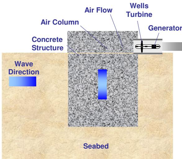
Figure 7: Oscillating water column type of wave device.
