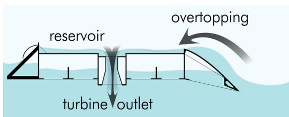
Figure 8: Overtopping type of wave device
