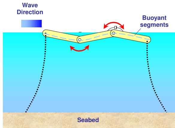
Figure 9: Pitching type of wave device.
