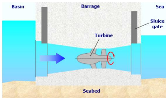
Figure 9: Tidal barrage type of tidal device.
