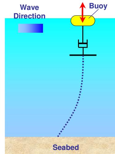
Figure 6: Buoy type of wave device.
