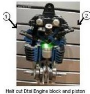
Fig.2. Cut section of Cylinder of Pulsar DTSI Bike
